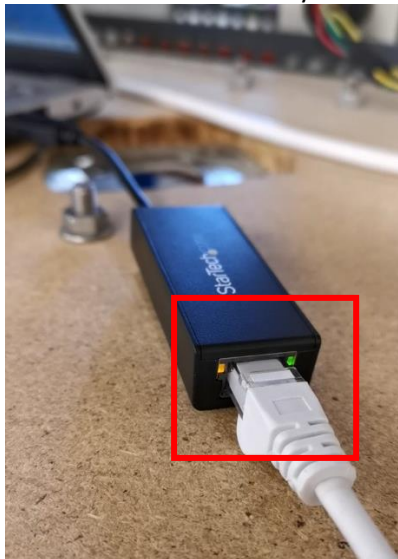
Figure 2 USB-Ethernet converter with LED indicator on and flashing
